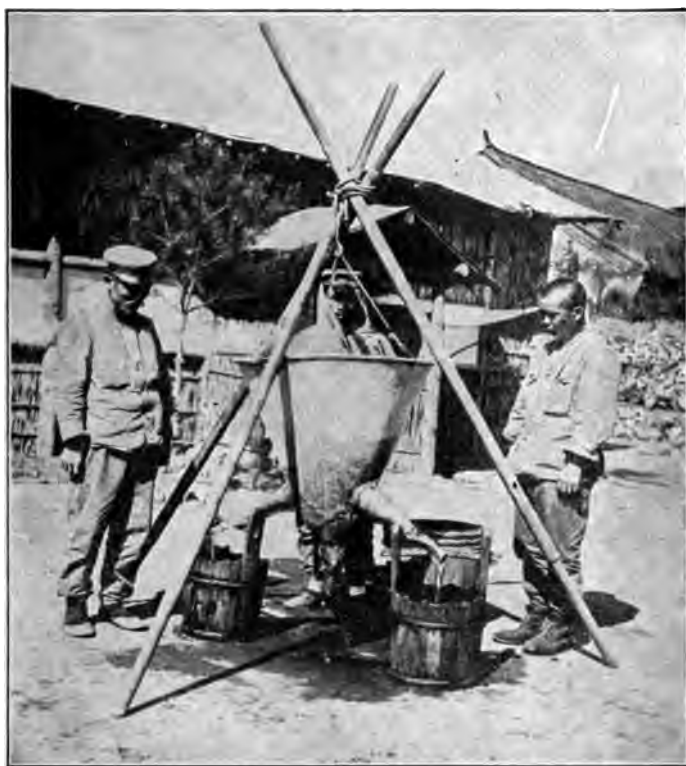
FIG. 62.—The Japanese field filter. ( Eshitzu filter. )
